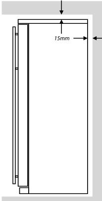
If located close to a corner adequate spacing must be left for door opening and removal of shelves. Refer to diagram.
